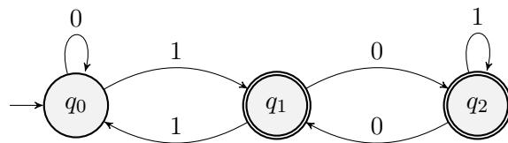
6a Write down the transition function  $\delta$  for this automaton.
